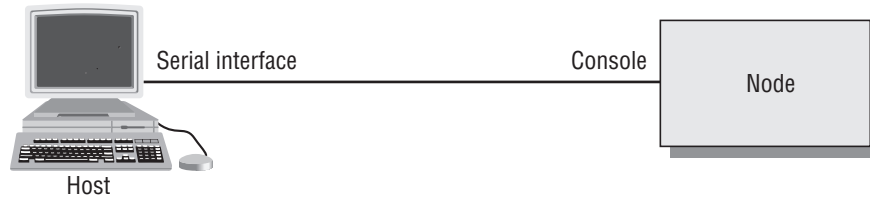
Figure 15. Setup for initial configuration via the console port
